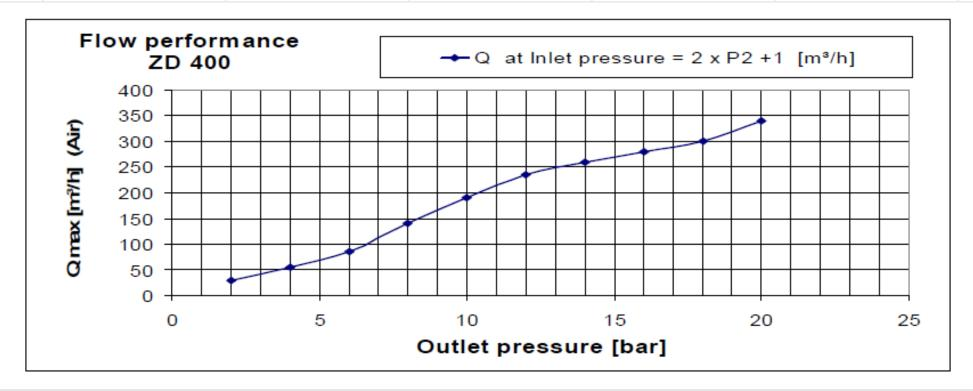
The pressure regulator ZD 400 reduces the max. inlet pressure of 300 bar down to a max. outlet pressure of 20 bar.
